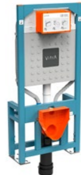
Regular wall-hung frame, 12cm, floor fixation with electrical & water connection, 3/6 litre H: 1120mm W: 500mm P: 200mm
