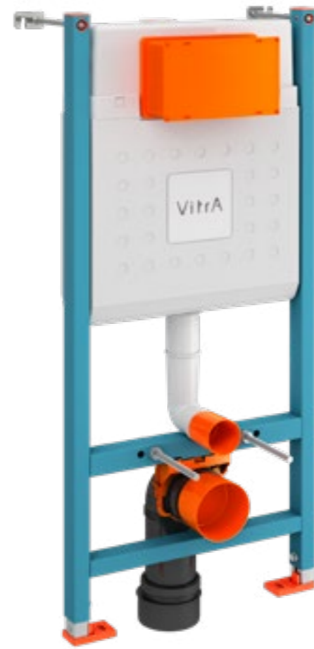
V-Fix Core wall-hung frame, 12cm cistern, 3/6 litre H: 1120mm W: 480mm P: 160-190mm
