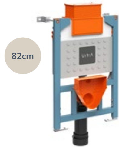
Reduced-height frame, floor & wall fixation, 82cm, 3/6 litre H: 820mm W: 500mm P: 160-190mm
