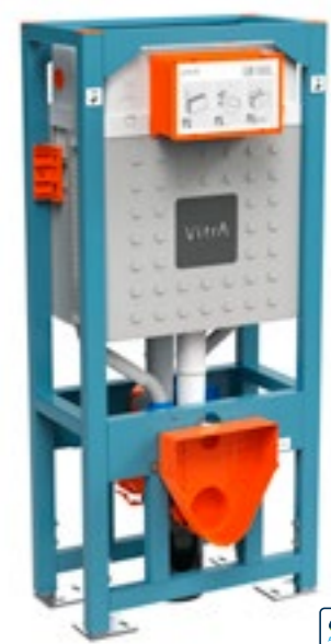
Regular wall-hung frame, 12cm, back-to-back double fixation with electrical connection, 3/6 litre H: 1120mm W: 500mm P: 260mm
