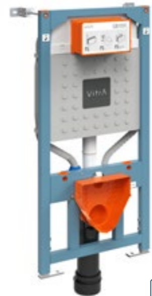
Regular wall-hung frame, 12cm, floor & wall fixation with electrical & water connection, 3/6 litre H: 1120mm W: 500mm P: 160-190mm
