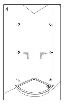
4 - Remove the assembly and drill the marked points using an 8 mm masonry drill bit, once this is done insert 6 x wall plugs into the holes.
