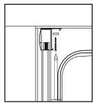
5 - Reposition the assembly and fix the wall channels to the wall using 6 x ST4x45 long screws (3 per channel)
