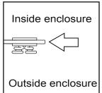
8 - Attach the handle making sure that the rubber washers that come with the handle are placed between the handles and the glass.
