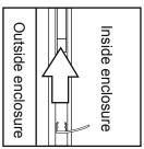
7 - Push the shorter 2 of the 4 water seals onto the exposed glass edges of the fixed panels, the flaps should face into the shower as illustrated.
