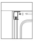
6 - Whilst ensuring that the bottom of the assembly is held snug to the shower tray and that all parts are level and upright, fix the assembly to the wall channels by drilling through the pre drilled holes in the wall channels into the profiles of the fixed panels using a 2.75 mm metal drill bit. Then secure using 6 x ST3.5x10 short screws (3 per wall channel).
